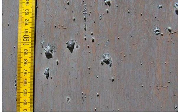
Fig. 9. Melt particles at containment wall
