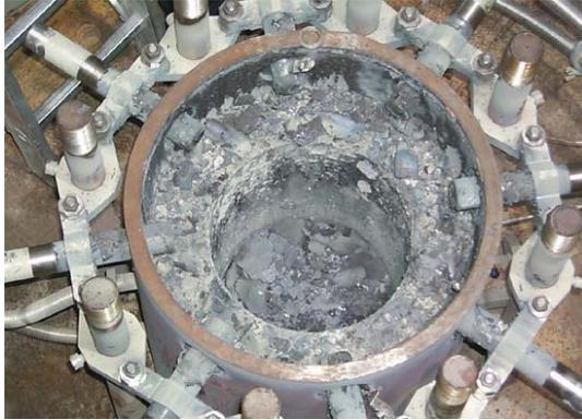
Fig. 8. Post test view of concrete cavity
