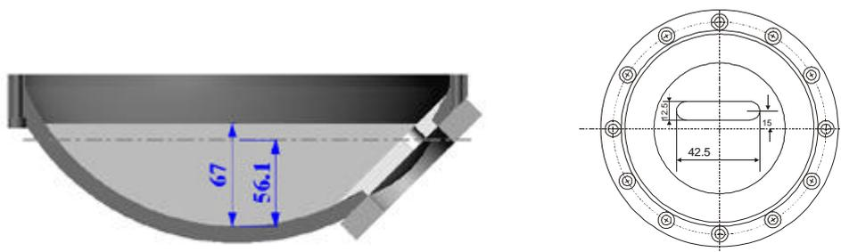
**Fig. 3** Geometry of lateral slot
